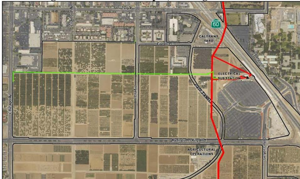
Aerial photograph shows UCR West Campus. The red line indicates the location of an existing 69kV subtransmission line. The green line is the location of a electrical distribution pole line.
